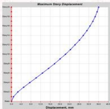
Storey Displacement Graph
